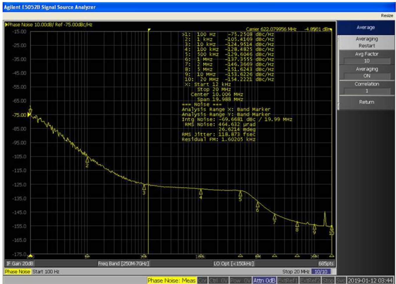
Figure 2. Representative Phase Noise Measurement: F_{OUT} = 622.08 MHz, F_{IN} = 10 MHz, BW = 100 Hz
