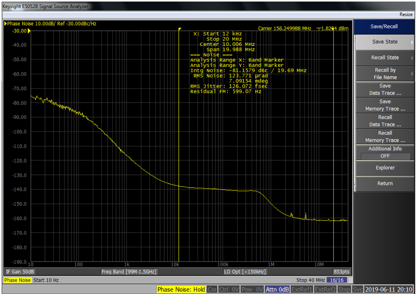
Figure 3. Representative Phase Noise Measurement: F_{OUT} = 156.25 MHz, F_{IN} = 10 MHz, BW = 100 Hz
