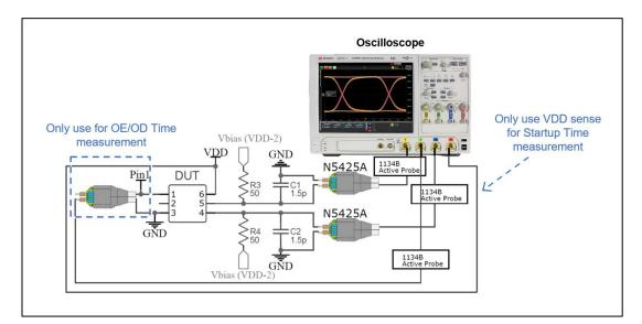
Figure 5. Test setup to measure LVPECL Waveform Characteristics, Current Consumption (with Termination 2)<sup>[14]</sup>, Output Enable/Disable Time, and Startup Time
