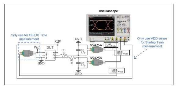
Figure 13. Test setup to measure Low-Power HCSL Waveform Characteristics, Current Consumption, Output Enable/Disable Time, and Startup Time
