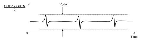
Figure 17. Differential Asymmetry (V\_da)
