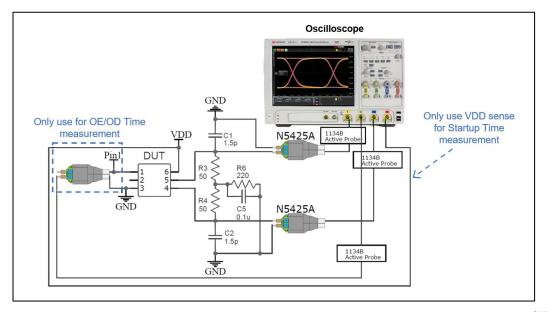
Figure 7. Test setup to measure FlexSwing Waveform Characteristics, Current Consumption<sup>[17]</sup>, Output Enable/Disable Time, and Startup Time
