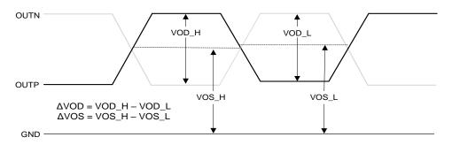
Figure 16. LVDS Voltage Levels per Differential Pin
