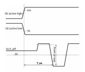
Figure 21. OE Pin Enable Timing (T\_oe)
