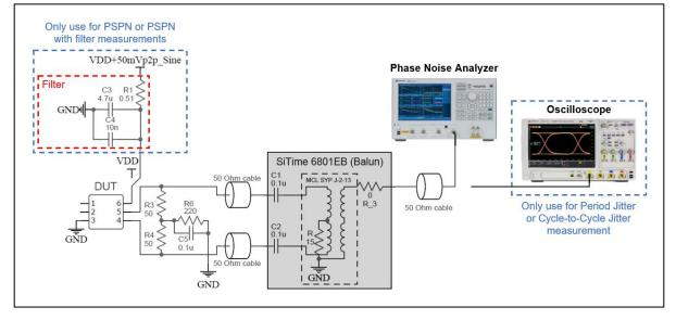
Figure 6. Test setup to measure FlexSwing Phase Noise, Period Jitter, Cycle-to-Cycle Jitter, and Power Supply-Induced Phase Noise (PSPN) with and without filter added<sup>[16]</sup>
