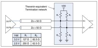
Figure 25. LVPECL and FlexSwing DC-coupled Load Termination with Thevenin Equivalent Network<sup>[19]</sup>
