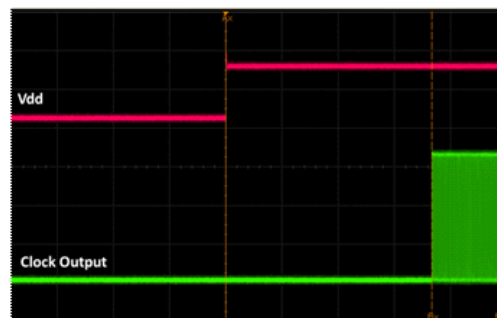
Figure 17. Startup Waveform vs. Vdd
