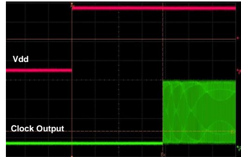
Figure 17. Startup Waveform vs. Vdd
